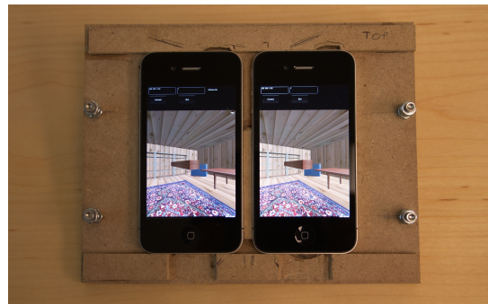
Figure 2: Experimental head mounted display with lenses removed, revealing the two smartphones that render and display imagery.
