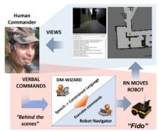
Figure 1: The Wizard-of-Oz experiment setup, where a human commander provides verbal instructions to a remote robot, given limited information from robot on screen (top). The robot is controlled by two wizards, one for handling NL and one for navigating the robot (bottom).
