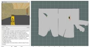
Figure 3: The Commander view in the simulated experiment setup with a Clearpath Jackal robot. The robot sends back images (top left), responds to instructions (bottom left), and displays a map (right).
