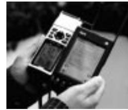
Figure 1: A Palm VII PDA with GPS receiver
