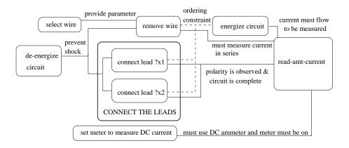
Figure 5: The BE&E Domain Plan for Measuring Current
