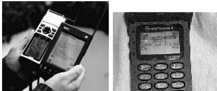
Figure 1. PDA (Palm VII) with GPS device and WAP-enabled cellular phone for wireless, handheld communication between proxy and user.
