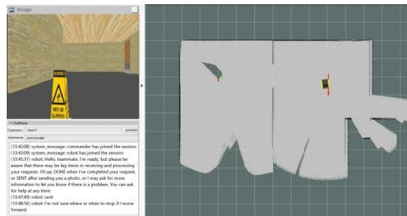
Figure 3: The Commander view in the simulated experiment setup with a Clearpath Jackal robot. The robot sends back images (top left), responds to instructions (bottom left), and displays a map (right).
