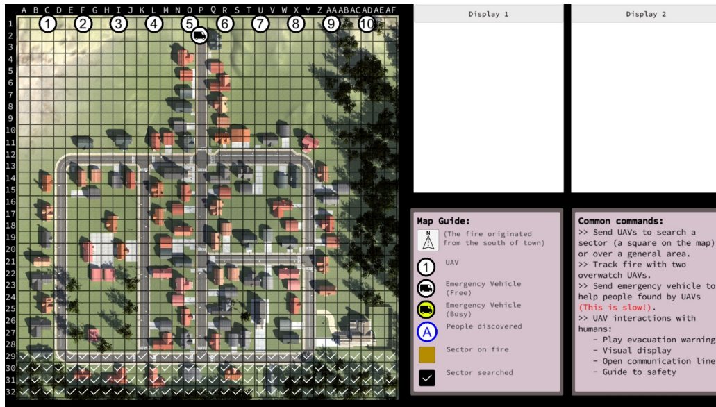
Figure 1. The operator's interface at the beginning of the simulation, showing the location of the ten drones and the rescue vehicle at the top of the map. Check marks at the bottom of the screen show areas that are known to be without residents. The map does not show the location of fire or any residents, because the drones have not yet been instructed to look for those.
