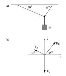
A block of weight W is suspended by strings (a). Consider the knot at the junction of the three strings to be the body. A free-body diagram shows all the forces acting on the knot (b). The strings are assumed to be weightless. The body remains at rest under the action of the three forces. Suppose we are given the magnitude of one of these forces. How can we find the magnitudes of the other forces?
